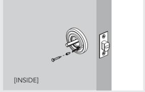
**M** Install supplied set screws into the inside and outside knobs or levers. Slide the nylon washers onto the base of the knobs or levers. From the interior side, push the spindle all the way in to remove any slack. Install outside knob or lever while pushing on the spindle from the interior. Secure the outside knob or lever with set screw.
