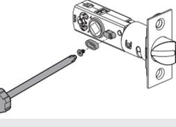
**F** Install latch using (2) #8 x 3/4 in (19 mm) screws.
