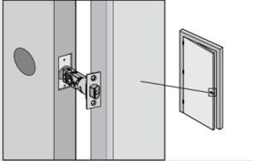
**D** While holding the latch to the door with the bevel side of the bolt facing the door frame, adjust the toggle to the upper L position for levers or the middle K position for knobs.
