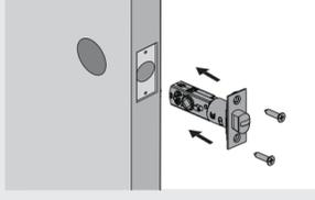
**G** From the interior side of the door, fully insert the long end of the spindle into the latch so the dog ears on the spindle are against the body and the groove faces down towards the lower hinge on both sides of the door.
