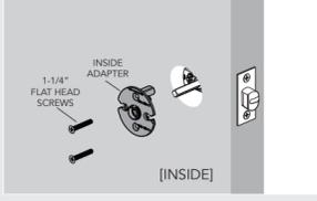
**J** Attach the interior and exterior roses with the hole in the rose facing the door latch and thread the retainer onto the adaptor. Securely tighten by using the wrench provided.
