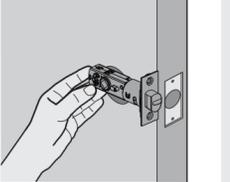
**B** Is the diamond shaped hole on the latch centered in the door hole? YES: Diamond shaped hole. No adjustment is required. Proceed to next step. NO: Diamond shaped hole. Rotate latch face as shown to extend latch.
