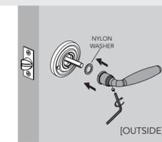
**N** Install the interior knob or lever. Secure the inside knob or lever with set screw.
