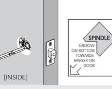
**H** Install the outside adapter with the words "Door Jamb" pointing towards the jamb where the strike will be installed. If using the spring-assisted adapter for levers, make sure the holder is attached. The spindle protrudes through the adapter.
