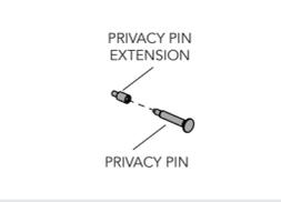
**L** Insert the privacy pin into the hole on the inside rosette towards the door edge and thread into the latch.
