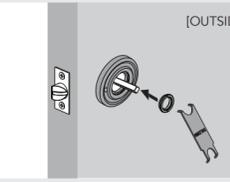
**K** If the privacy latch set is being installed on a door 1-3/4 in (44 mm) thick add the privacy button extension before proceeding.
