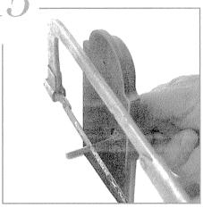
Cut the thumbturn tailpiece so that it goes half way through the lock. (as in step 12)
