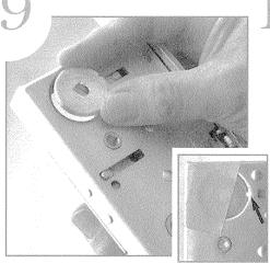
Thread the cylinder plug into interior side of lock. Place a strip of tape over plug to keep it from turning. Notch must be located as shown. (Double cylinder functions: OMIT THIS STER.)
