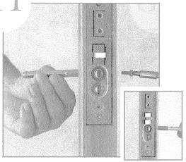
For handleset trim install the spindle from the inside with V groove facing bottom door hinge and thread the screw and lock washer into the spindle from the outside. Tighten securely. For knob to knob and lever to lever sets, install spindle from outside - go to step 13.
