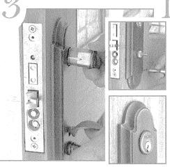
Place the cylinder through the trim. Partially insert key into cylinder. Thread the cylinder into the lock until it is against the trim and Baldwin name is horizontal. For knob to knob and lever to lever sets - Install aligning bushing and fasten trim with supplied screws. Remove bushing - go to step 16.
