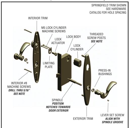
**#8 Machine Screws Note:** Proper trim alignment requires installing the spindle and levers before completely securing the #8 screws.
