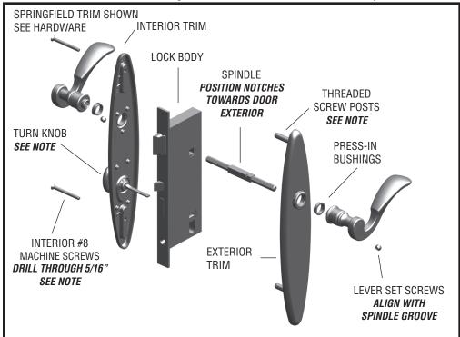
**Turn Knob Note:** Shown is the lever on the top of the turn knob. The lever may be on the bottom, depending on the lock. **#8 Machine Screws Note:** Proper trim alignment requires installing the spindle and levers before completely securing the **#8** screws.
